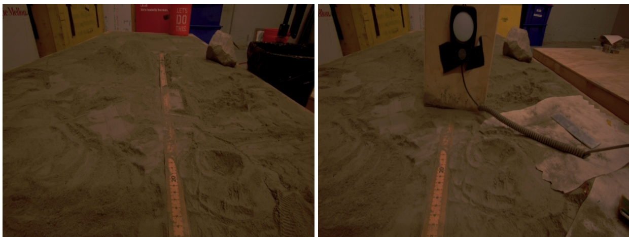
Figure 5.1. Scenes for Testing Illumination. A cement-powder scene with a small crater in front and a rock far away was used for illumination testing. Cement powder served as an optical
