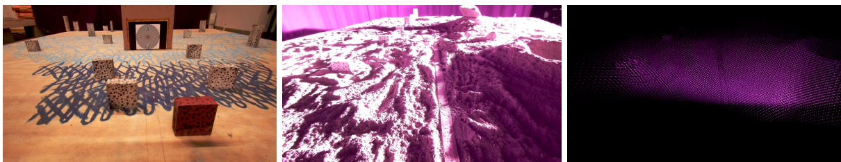
Figure 6.8. Test Case Datasets. Three datasets were used to evaluate the accuracy of the stereo pipeline, disparity maps generated by stereo matching, and point clouds generated by depth calculations. The three datasets each tested a unique environment. Left: The “Blocks World” dataset tests an environment of fixed geometry. Center: The “Lunar Sunlight” dataset comprised lunar analog terrain illuminated at lunar polar sunlight intensity approximating solar spectral distribution. Right: The “Dot-Illuminated” dataset comprised lunar analog terrain illuminated by laser dot projectors, what a rover would perceive in the shadows characteristic of the poles.
