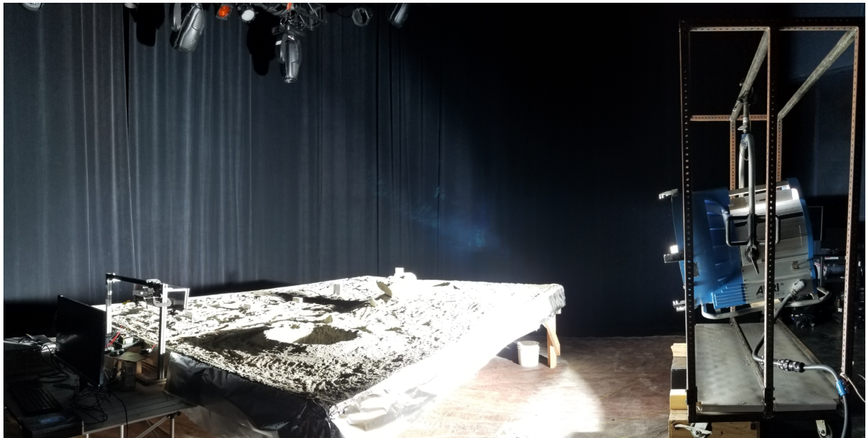
Figure 4.1. Simulating Lunar Lighting on Lunar Terrain. Arrimax 18/12 cinematic light [31] projecting 18 kilowatts of “sunlight” onto MoonRanger’s perception testbed.
