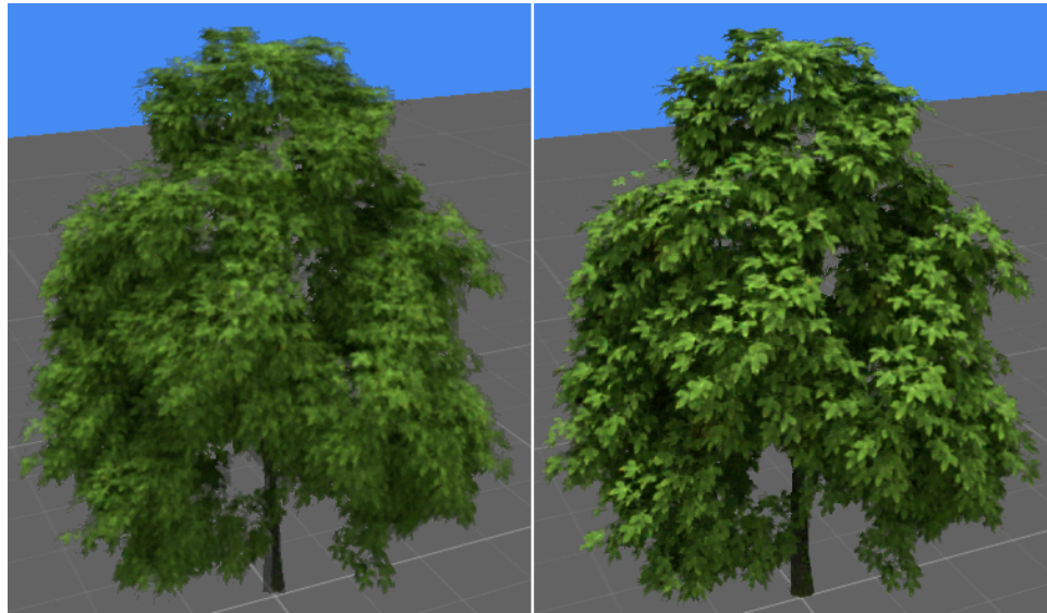
Figure 5.4: When nearest color rays are interpolated to produce a final image, the blending of multiple views results in ghosting artifacts (left). Using depth data to interpolate between rays that strike a particular point on the model eliminates nearly all of these artifacts (right).
