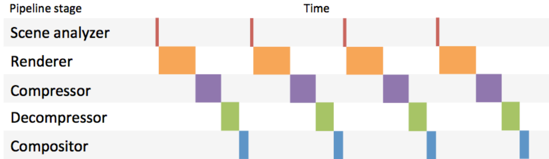
Figure 4.3: An example timeline showing active pipeline stages when there is only one frame in the pipeline at any given time. Sending only one frame at a time severely underutilizes all stages and results in a lower frame rate. Stages that take negligible time, such as frontend request sender, backend request receiver, etc., have been removed to simplify the figure.
