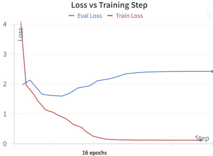
Figure 4.3: Full memorization evaluation and training losses. Training loss stabilizes at 16 epochs, but evaluation loss hints at overfitting.
