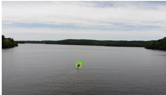
Figure 2.3: Drone using object detector to search for people over water
