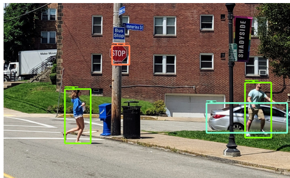
Figure 2.1: Autonomous vehicle using object detector to detect traffic signs and pedestrians on the road
