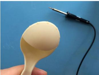
Step 5: Solder cover to create watertight seal Using a gentle back and forth motion, solder the cover in place. Make sure you penetrate deep enough so that the weld will hold after sanding. But be careful not to solder too deep or your final spoon will look ragged even after sanding.
