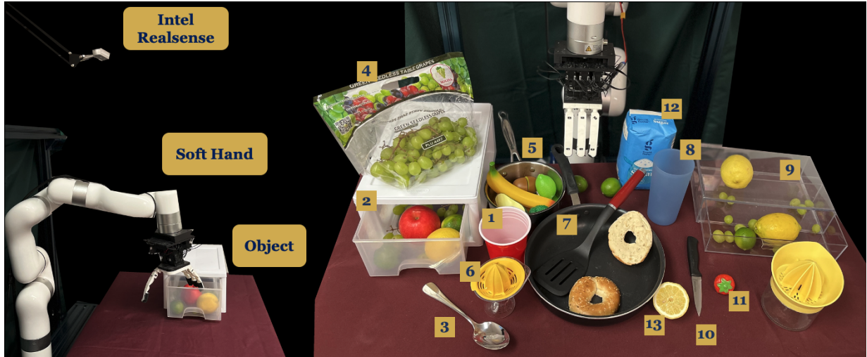
Figure 2.4: Left: Workspace Setup. We place an Intel RealSense camera above the robot to maintain an egocentric viewpoint, consistent with the affordance model’s training data. Right: Thirteen objects used in our experiments.
