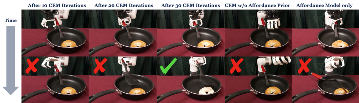
Figure 2.6: Qualitative results showing the finetuning procedure for DEFT. The model learns to hold the spatula and flip the bagel after 30 CEM iterations.
