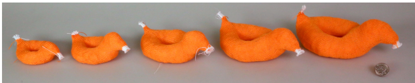
Figure 4.1: A row of knit ducks of different sizes created directly from a 3D mesh and a scaling factor. This pattern was constructed seamlessly in one piece by the knitting machine and stuffed in post-process.
