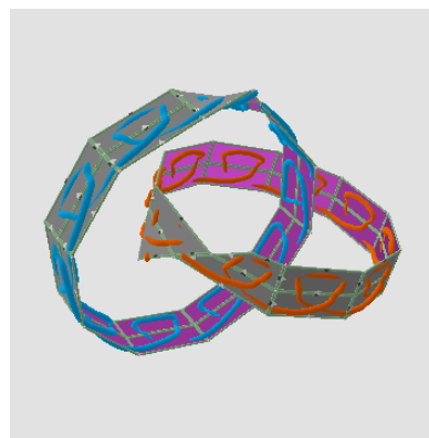
Figure 5.6: A smobj with linked cylinders as shown here does not have an embedding that is both intersection free and monotonic. Note that a surface with this topology can be constructed with a different stitch mesh.
