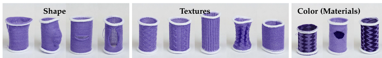
Figure 2.15: Knit shapes can be edited in various ways. Its shape can be changed by increases (decreases) and short-rows. Textures can be edited by using increases and decreases to create lace work, cables and knit-purl variations. Multiple materials can be introduced to edit the structure in various techniques like plating, intarsia and fairisle style knitting
