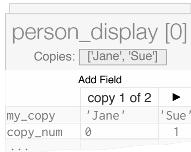
Figure 4.15 An object with multiple copies; copies is set to ['Jane', 'Sue']. Every copy has two properties: my_copy , which is set to that copy's item (here, either 'Jane' or 'Sue') and copy_num , which is set to that copy's index. Here, we are looking at the first copy (index 0).
