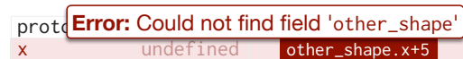
Figure 4.17 Syntax and runtime errors are highlighted in the editor but do not prevent the program from running. Fields with errors and other fields that depend on them are given the value undefined .
