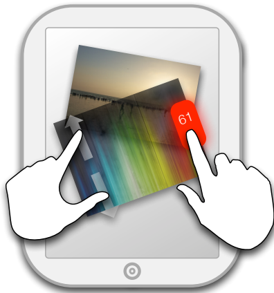
Figure 3.10 An illustration of a touchscreen-based application written with ConstraintJS. Constraints control the position, scale, and angle of photos, which users can manipulate with one or two fingers. When two fingers touch a photo, a red slider appears that controls the photo's opacity and can be changed using a third finger. Constraints set the position and text of the slider.
