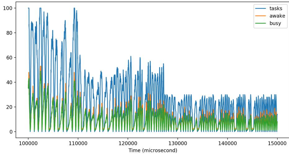
Figure 4.6: Profiling for the `prime` benchmark problem from 50ms to 100ms and 150ms to 200ms. Instantaneous parallelism varies dramatically and exhibits burstiness in both sections. From 150ms to 200ms, the computation has limited parallelism.
