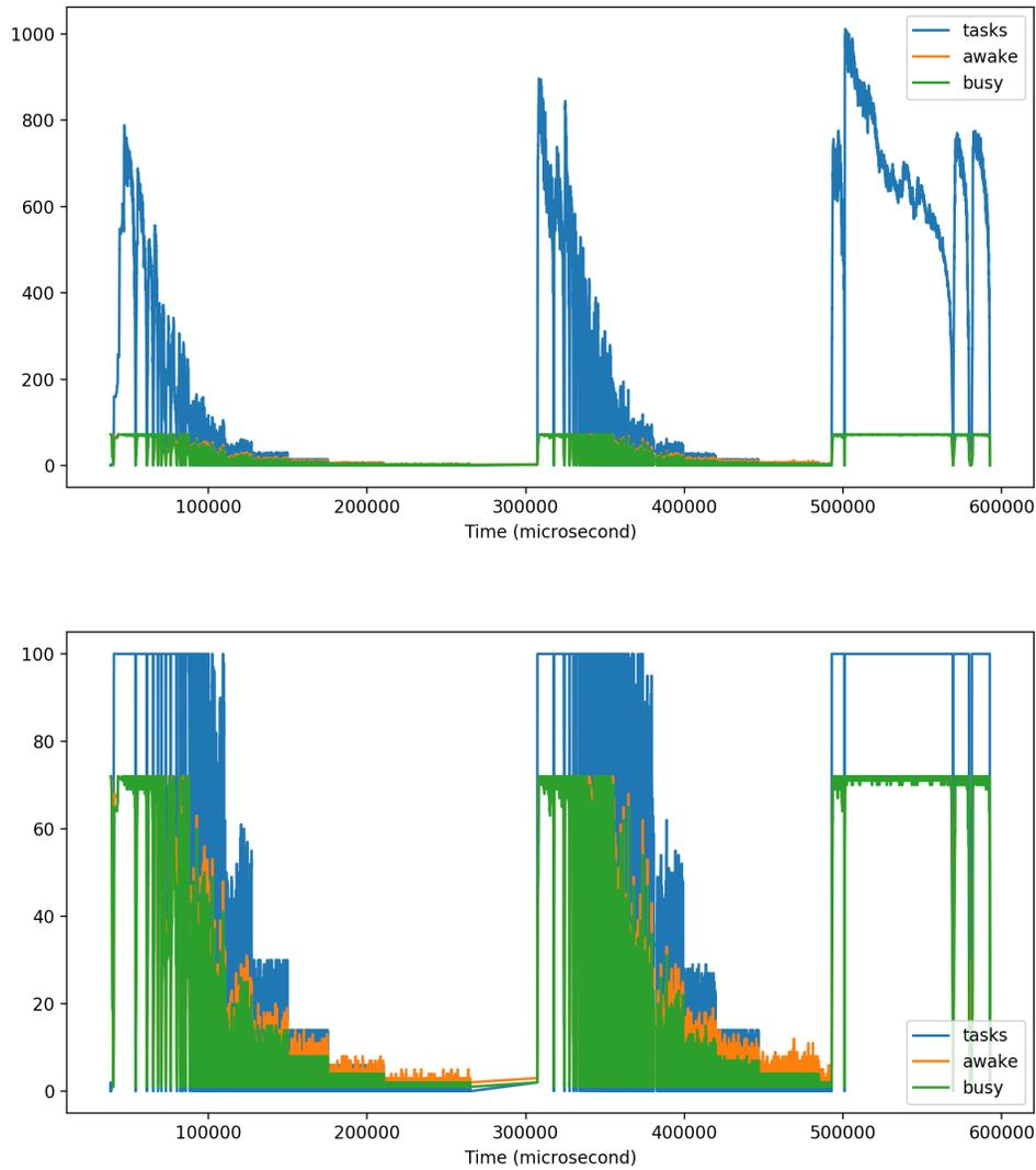
Figure 4.5: Profiling for the `prime` benchmark problem. The `tasks` curve shows the number of tasks in the system. The `awake` curve shows the number of active processors in the system, and the `busy` curve shows the number of processors working on actual computation. In the second subfigure, we trimmed the Y-Axis by 100 because we are mostly interested in the behavior of our algorithm in the face of low instantaneous parallelism.
