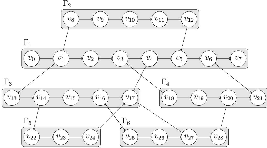
Figure 1.1: An exemplary computation dag  $G$  consisting 6 thread  $\Gamma_1 \dots \Gamma_6$  and 28 nodes  $v_1 \dots v_{28}$ .  $v_0$  is the *root* and  $\Gamma_1$  is the initial thread. Computation starts with node  $v_0$  in  $\Gamma_1$  and terminates with  $v_7$  in  $\Gamma_1$ . For this graph,  $T_1 = 29$ , and the span  $T_\infty = 14$ .
