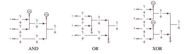
Figure 9: AND, OR, XOR circuits using diode-resistor logic and intermediate molecular latches.
