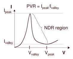
Figure 2: I-V curve for a "typical" RTD device.
