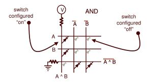
Figure 1: A two-input AND gate implemented in a reconfigurable CAEN grid.
