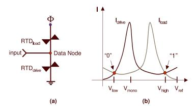
Figure 3: (a) Basic molecular latch configuration. (b) Load-line diagram for molecular latch.
