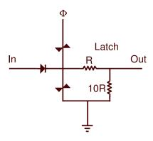
Figure 8: The complete molecular latch.
