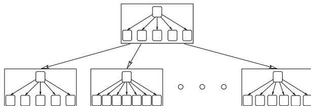
Figure 27: fpB<sup>+</sup>-Trees for variable length keys
