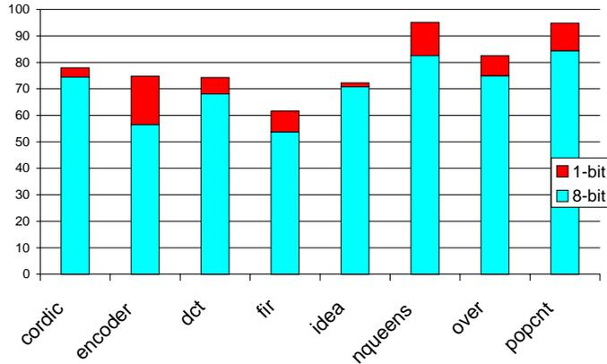
Figure 6: *Percent of the hardware removed by BitValue when synthesizing programs for reconfigurable hardware devices; the bottom bar shows savings when using 8-bit wide processing elements, and the top bar when using 1-bit wide processing elements.*
