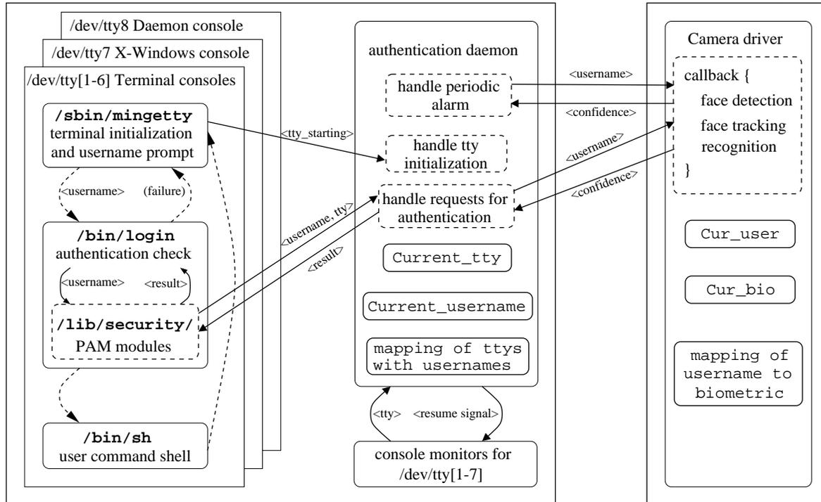
Figure 2: Implementation of Continuous Video Enhanced Authentication System
