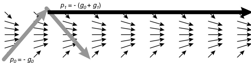
Figure 7.2: The Conjugate Gradient Method Escaping a Trough
