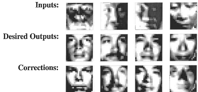
Figure 2.17: Architecture for correcting the lighting of a window. The window is given to a neural network, which has a severe bottleneck before its output. The output is a correction to be added to the original image.
