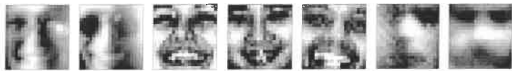
Figure 2.13: The steps in preprocessing a window. First, a linear function is fit to the intensity values in the window, and then subtracted out, correcting for some extreme lighting conditions. Then, histogram equalization is applied, to correct for different camera gains and to improve contrast. For each of these steps, the mapping is computed based on pixels inside the oval mask, and then applied to the entire window.
