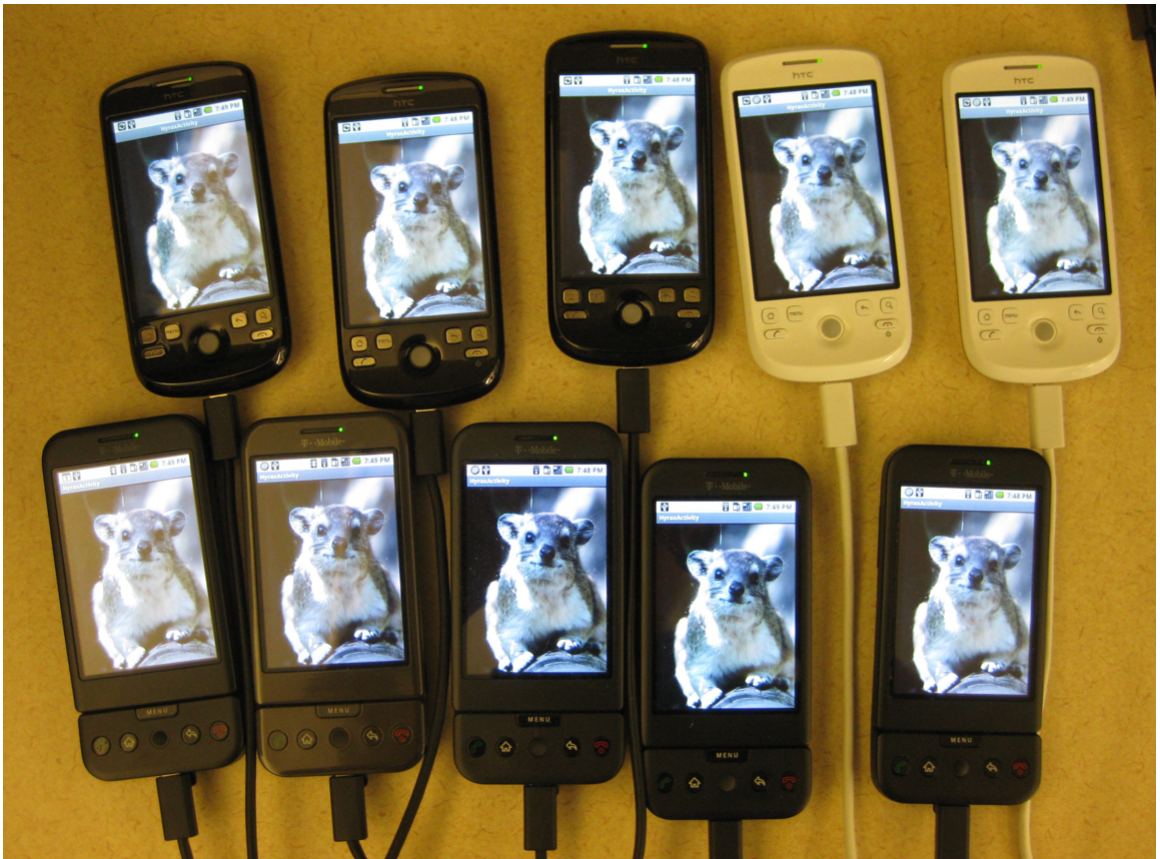
Figure 6.1: Hyrax workers running on our Android smartphone cluster.
