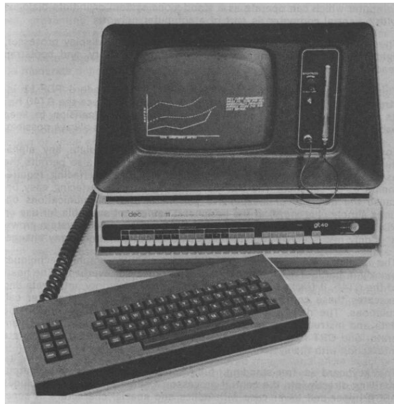
Figure 2.2: A DEC GT-40 terminal, introduced in 1972, features many of the same I/O capabilities as Sutherland's Sketchpad system including vector-based graphics and a light pen input device. Image from the 1976 PDP-11 Peripherals Handbook, as appears at http://www.brouhaha.com/eric/retrocomputing/dec/gt40/handbook.html .
