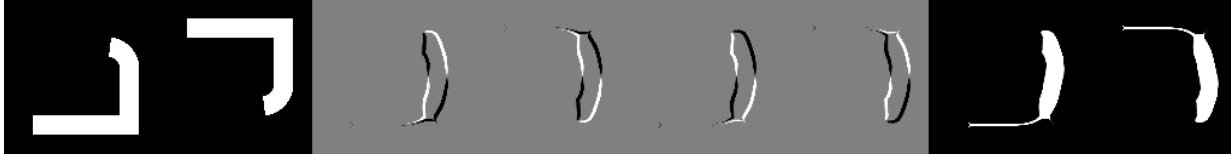
Figure 3.6: Oscillation in the simplified Christensen-Rabbit-Miller algorithm due to its Euler integrator with a fixed step size. The two shape images on the left, the source and the target images, are interpolated using an exaggerated step size of 0.25. The second panel shows the difference between the deformed source during interpolation iterations 10 and 11 while the fourth shows the difference between the same for iterations 9 and 10. The third and fifth panels show analogous images for the target. The deformed source and target for iteration 11 are shown in the rightmost two panels. The deformations for iterations 10 and 11 are essentially each other's inverse, indicating oscillation.
