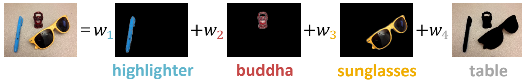
Figure 1.1: Many tasks within computer vision can be posed as decomposing an image into its constituent parts. In the task of semantic segmentation, pixels are grouped into non-overlapping parts that correspond to different objects within a scene. Even without extensive supervision, prior knowledge such as object color consistency can encourage more accurate segmentations.
