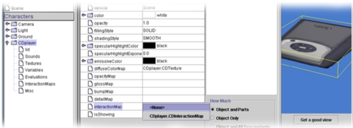
FIGURE 5-15: The designer can make any interaction map assigned to an object its active interaction map.
