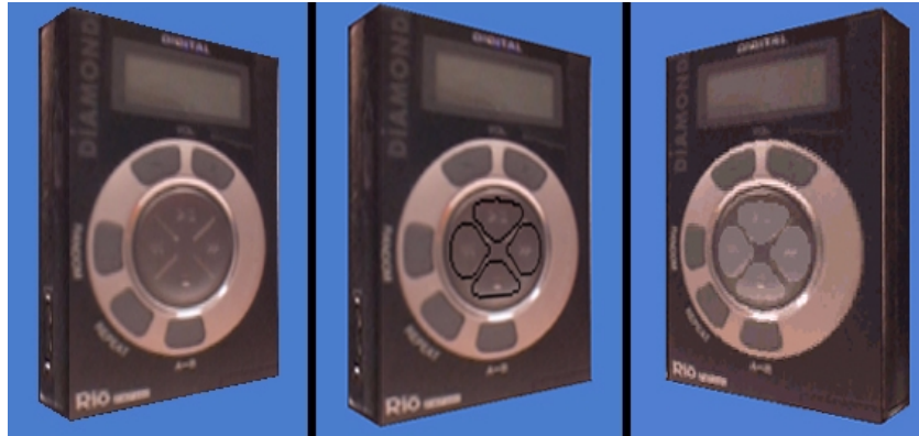
FIGURE 5-16: The MP3 player (left) with feedback textures showing the outlines of interaction surfaces (middle) and lighter areas corresponding to the interaction surfaces (right).
