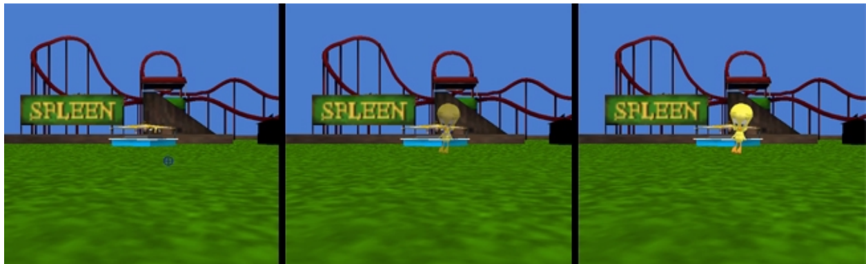
FIGURE 3-17. When the user positions the crosshair over an object the system provides feedback by creating a transparent doll for the object. The doll turns opaque when the user pinches his fingers together.
