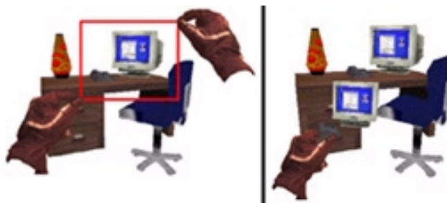
FIGURE 3-3. A user can explicit specify the context by framing the desired objects on his image plane.
