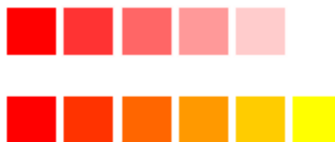
FIGURE 5-11: Color tiles with constant hue and equally distributed saturation (top) appear to be a single color that fades away, while color tiles with constant red values and equally distributed green values (bottom) appear to be different colors.
