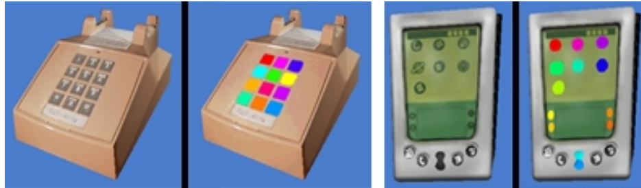
FIGURE 5-3: Designers can paint interaction maps for both photogrammetric models (left) and hand-painted models (right) to allow users to interact with parts of the models only present in their textures.
