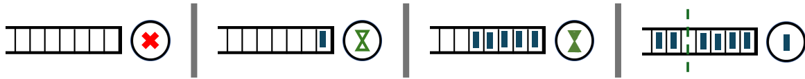
Figure 1.2: A comic illustrating of the indirect nature of setup (Section 1.2.1). In the first panel, the queue starts empty. Then, a job arrives triggering the setup of the server. While the initial job is waiting for the server to turn, more jobs arrive, all observing the server in setup—the main cause of their delay. However, jobs which arrive after the server is ready still experience additional delay—but do not directly observe why they are delayed.
