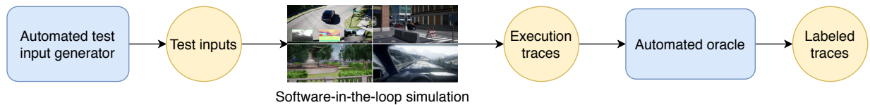
Figure 1.1: Automated testing pipeline for a cyberphysical system using simulation. An automated test input generation technique (Chapter 5) creates test inputs that will be executed on the CPS in simulation, which results in execution traces. These traces are provided to an automated oracle (Chapter 4) to be labeled as either correct or erroneous.
