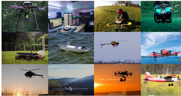
Figure 2.1: A variety of cyberphysical systems, including airplanes, helicopters, and submarines, that use ArduPilot as an autopilot software. (Source: https://ardupilot.org )
