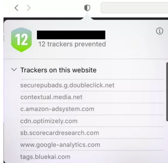
Figure 3.9: Safari offers a dashboard that displays information about blocked trackers, but offers no controls. Some limited controls are available elsewhere, in the main browser settings.
