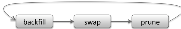
Figure 6.2: The round-robin strengthening strategy performs one backfill, one swap and one prune, repeating until no more strengthening actions are possible.
