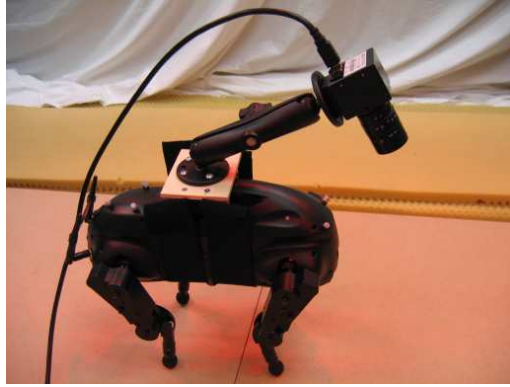
Figure 5.1: Firewire camera attached to LittleDog via boom on saddle.
