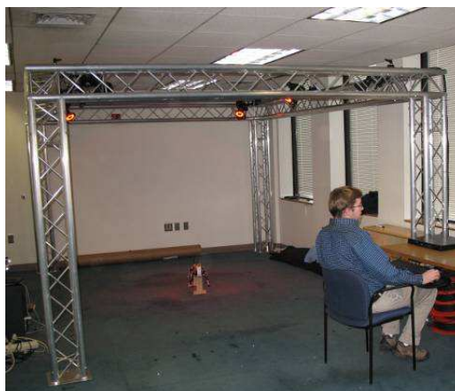
Figure 1.3: The frame of the motion capture system within which the dog must remain for it to operate. Copyright Boston Dynamics.
