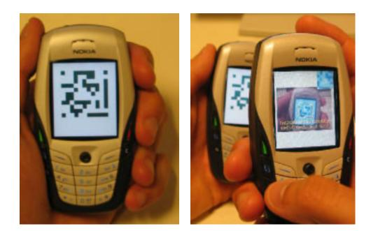
(a) SiB application displaying a hash encoded in a barcode.
