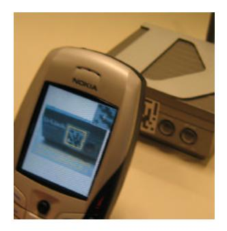
Figure 3: Phone running SiB scanning a barcode on an 802.11 wireless base station.
