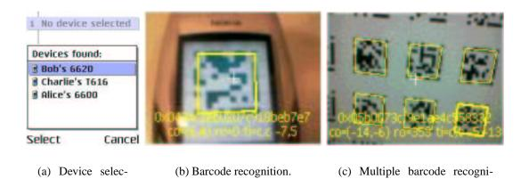
Figure 4: Mobile phone screen shots showing the SiB application in operation. In the first screen shot, the user is being prompted to select a device with which to initiate the SiB protocol. In the second, the user sees the phone at which he is aiming his camera, with status markers indicating successful barcode recognition. The third image is successful recognition of multiple barcodes displayed on an LCD screen.
