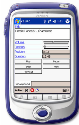
Figure 2.3. An interface generated for WinAmp on a PocketPC using the INCITS/V2 framework [IMTC 2006]. Reproduced with permission.
