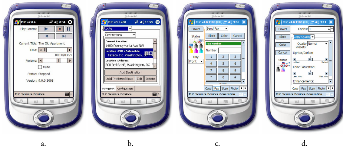
Figure 1.2. Interfaces generated by the PUC on the PocketPC for several different appliances: a) Windows Media Player 9, b) the navigation system from a 2003 GMC Yukon Denali, c) the Canon PIXMA MP780 all-in-one printer, and d) the HP 2610 all-in-one printer.
