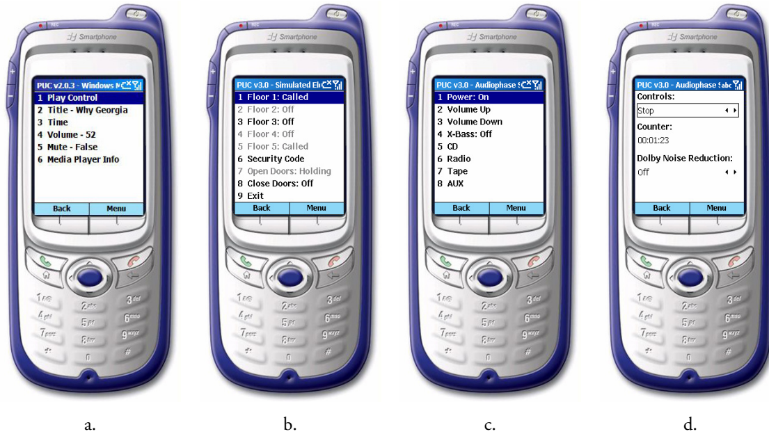
Figure 1.3. Interfaces generated by the PUC on the Smartphone for several different appliances: a) Windows Media Player, b) a simulated elevator, c-d) a shelf stereo with CD, radio, and tape functionality.
