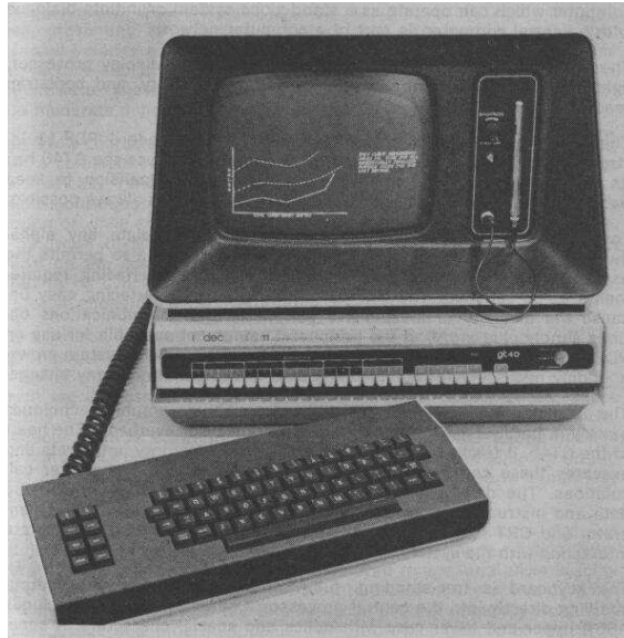
Figure 2.2: A DEC GT-40 terminal, introduced in 1972, features many of the same I/O capabilities as Sutherland's Sketchpad system including vector-based graphics and a light pen input device. Image from the 1976 PDP-11 Peripherals Handbook, as appears at http://www.brouhaha.com/eric/retrocomputing/dec/gt40/handbook.html .
