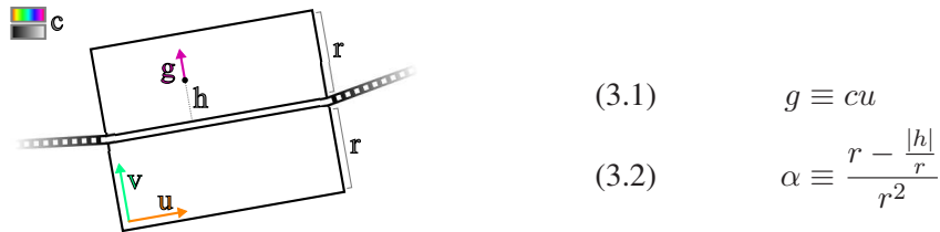
Figure 3.7: The desired gradient at a given position a gradient brush stroke is the perpendicular vector to the spine multiplied by the current color. The blending weight at a given position increases linearly to the stroke’s spine and is normalized by stroke radius.
