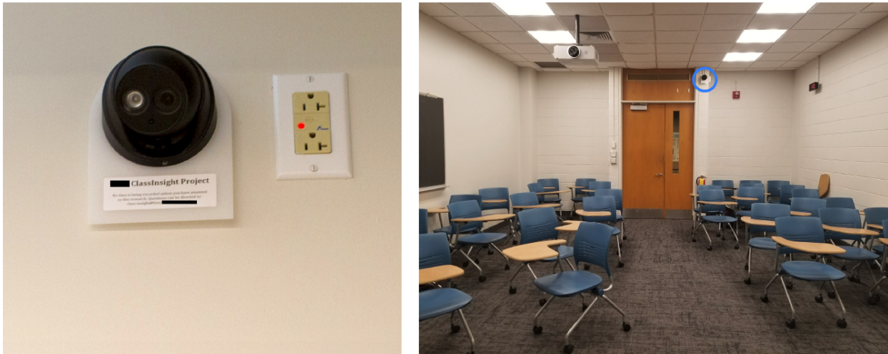
Figure 7-1: (On the left) Sensor consisting of a camera that collects audio and video data. (On the right) Sensor installed at the back of the classroom, facing the front, to collect audio and video data on the instructor.
