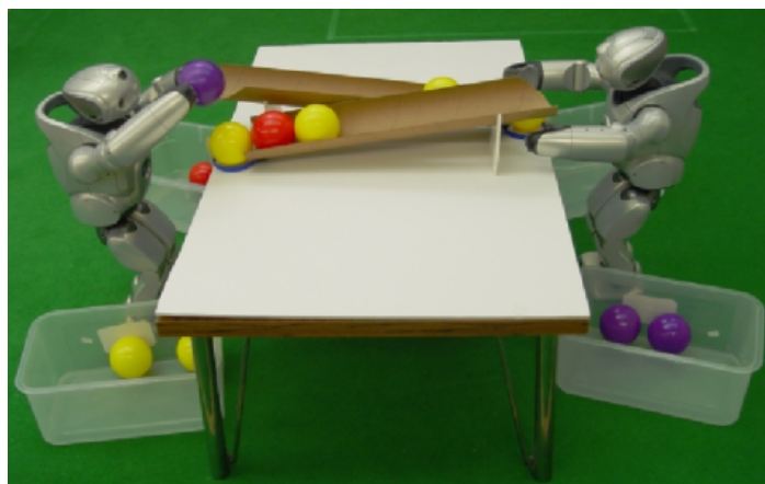
Figure 6.1: QRIO robots performing ball sorting task.
