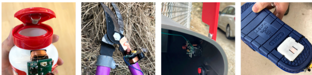
Figure 5.1: Four Sozu-augmented objects that use motion energy: pill bottle, garden pruner, mailbox, and slipper
