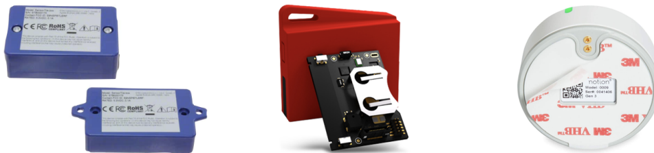
Figure 2.2: Examples sensor tag products, from left to right: STMicroelectronics SensorTile [16], TI SensorTag [17], and Notion multi-purpose sensor tag [24].
