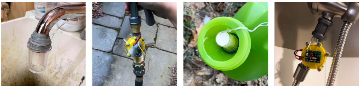
Figure 5.7: Sozu can be powered by the flow of water from a sink faucet, garden hose, watering can, and showerhead.
