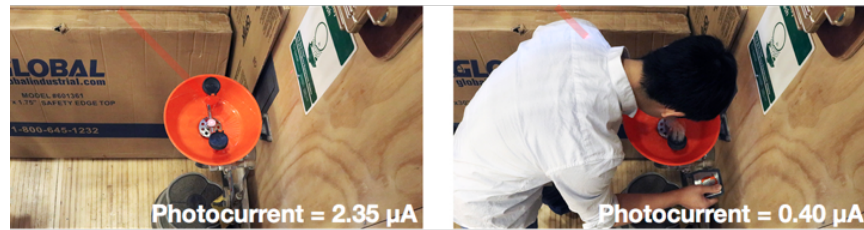
Figure 6.18: Tag occlusion is easily detected by measuring the reflected light intensity, and can be used to infer use.
