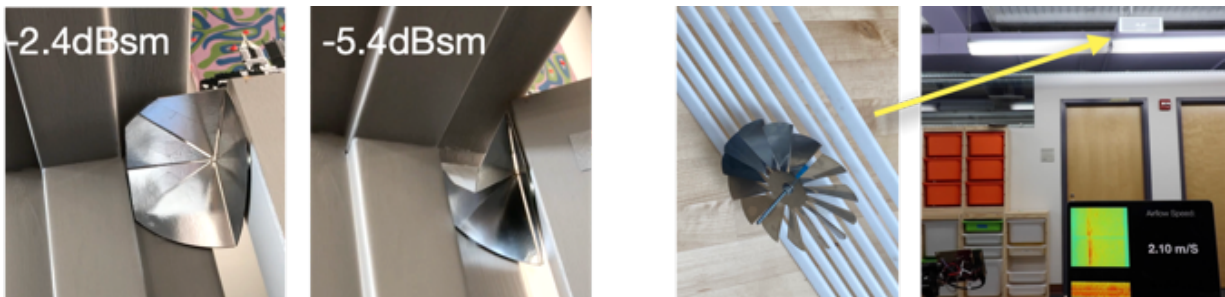
Figure 7.7: Two dynamic reflector mechanisms designed for door state detection (left) and HVAC airflow sensing (right).
