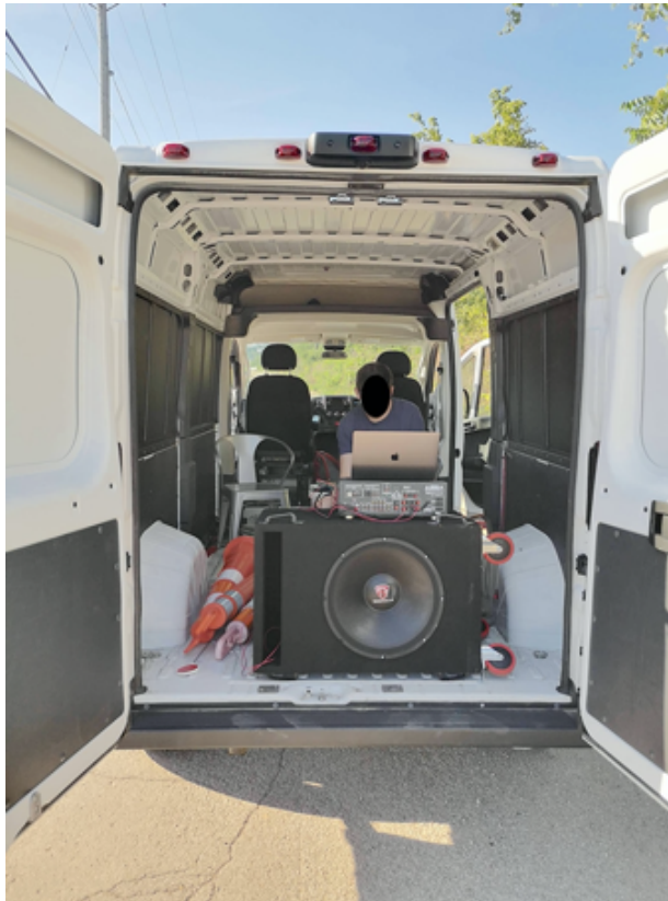
Figure 8.9: We loaded our signal generation apparatus into a van for mobility, which allowed us to test various distances in outdoor conditions.
