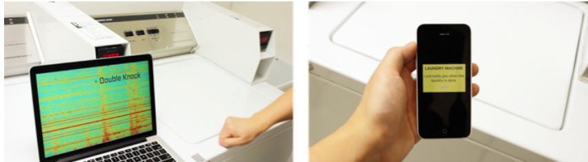
Figure 6.16: A user double knocks on a laundry machine to request a completion notification.
