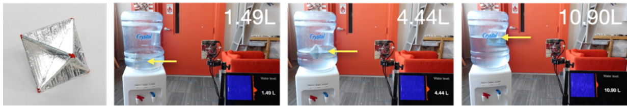
Figure 7.6: Tracking a sensor that floats at the water level for monitoring the amount of water left in the dispenser.
