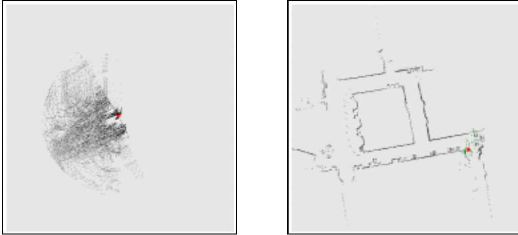
Figure 8: Mapping without odometry. Left: Raw data, right: map, generated online.
