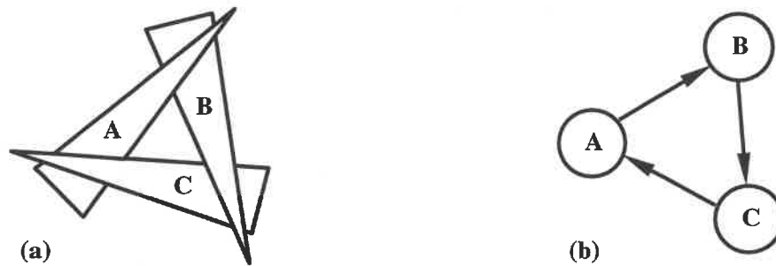
Figure 3.12: (a) A configuration of three objects and (b) its associated cyclic occlusion graph.
