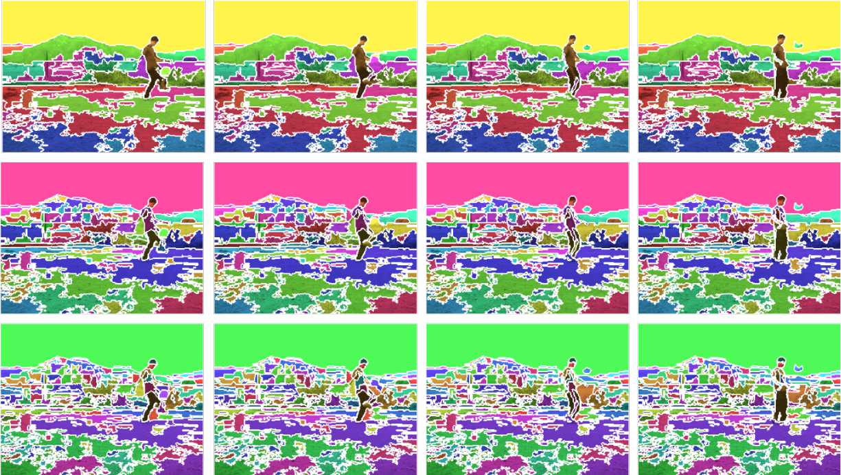
Figure 4.3: Three levels of segmentation hierarchy generated by the streaming GBH [105] algorithm. The top row shows the highest, most coarse level, while the bottom row shows the finest level of segmentation.
