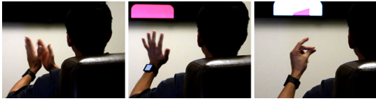
Figure 5-13. Gestures can control remote devices. In the left, the user claps to turn on the TV. Wave gestures navigate and snaps select.
