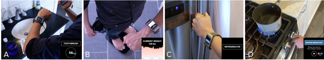
Figure 4-6. EM-Sense can augment activities in the home. For example, EM-Sense can launch a timer (inset) when the user is brushing his teeth (A), or display the user’s data when stepping on a scale (B). Next, EM-Sense knows that the user is making breakfast and fetches the morning news (C and D).
