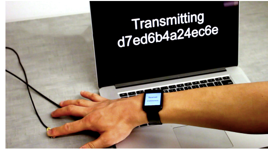
Figure 5-7. We implemented a range of encoding schemes to robustly transmit data-encoded vibrations.
