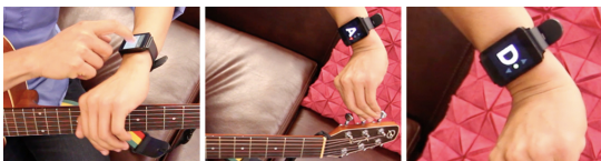
Figure 5-15. For an unpowered object e.g. , an acoustic guitar, we can detect the closest note to tune the instrument precisely.
