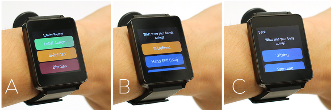
Figure 6-1. The experience sampling watch app. At random intervals, wearers are prompted for activity labels (A), after which they select a hand activities (B,C).
