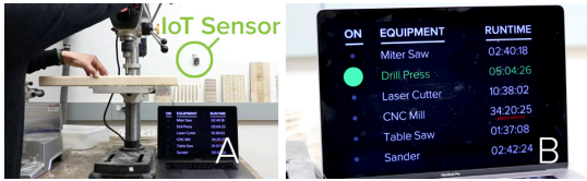
Figure 12-12. IoT sensors could track equipment use (A) for safety and maintenance (B).
