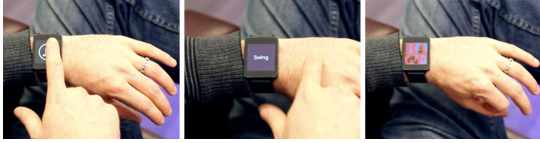
Figure 5-11. In a launcher, we can place navigation controls on the skin. Users can traverse back up through the hierarchy with a flick gesture.
