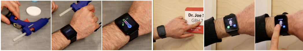
Figure 5-17. Vibro-tags emit structured vibrations that carry data. For example, the user can touch an office nameplate instrumented with a vibro tag (top), which transmits the person's contact details to the smartwatch. We can also instrument non-mechanical objects, e.g., a glue gun (bottom). It broadcasts an object's ID and metadata — in this case, the current temperature and ideal operating range.
