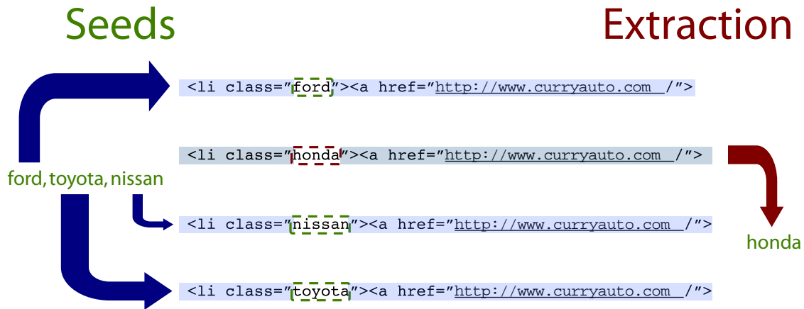
Figure 4.1: An illustration of wrapper induction. Seeds are located in a retrieved document, a template consisting of a prefix and a suffix is found, and new candidate instances are extracted using the template.
