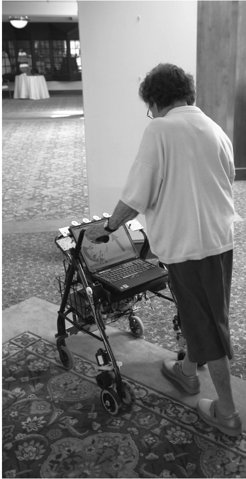
Figure 6. Using the Location System. Note the buttons located along frame above laptop screen
