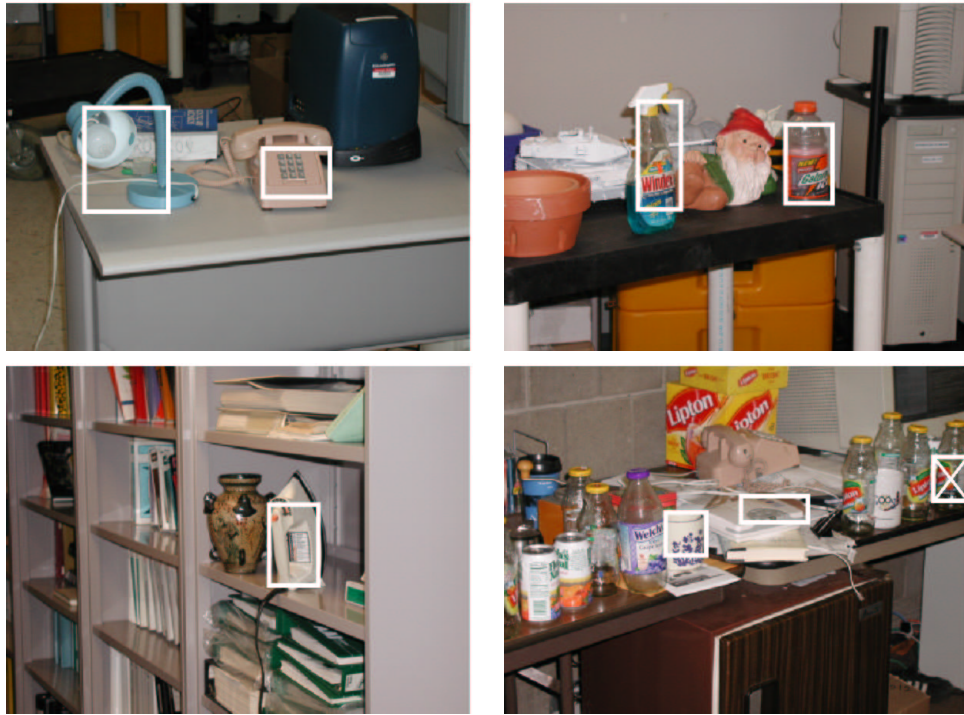
Figure 7.9: Anecdotal results with more than one object of interest per test image. Correct detections are shown as empty white boxes while false positives are shown as crossed boxes.
