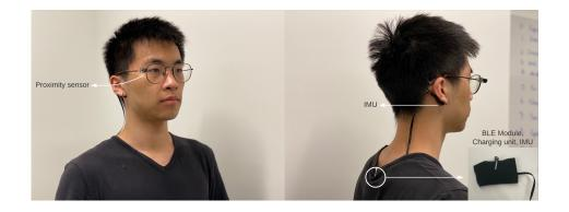
Figure 6.3: FitNibble wearable setup. The system has a proximity sensor to detect hand-tomouth gestuers (left), an IMU in contact with the lower jaw bone to detect chewing (right), and small cloth pocket clipped to the back of the user's shirt containing the BLE module, battery, and the reference IMU (bottom right)
