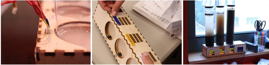
**Figure 6.6. Designing a bio-electronic system: column plugged into casing; labeling the column slots; testing the system.**
