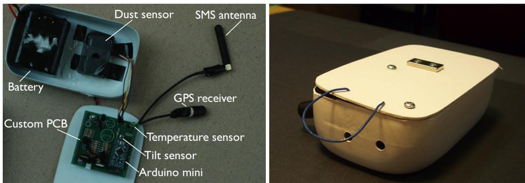
**Figure 3.7. Dust sensor in case with parts labeled; back of case with magnet and strap.**
