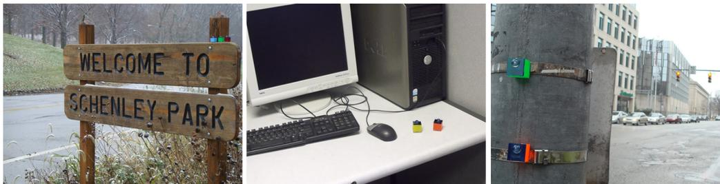
**Figure 3.5. Student sensor placements: exhaust, chemicals and smog on park entrance sign; noise and exhaust at bus stop; dust and noise sensors in computer lab.**
