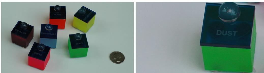
**Figure 3.1. All six sensor probes (left) and dust probe (right).**
