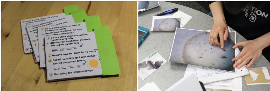
**Figure 6.2. Particulate matter traps, ready to be mailed to participants, and participant examining microscope image of collected particles during community workshop.**
