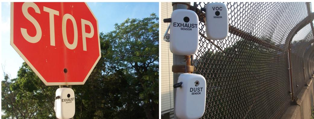
**Figure 3.6. Functional place-based sensors: exhaust sensor attached to stop sign; dust, exhaust and VOC sensors attached to bridge.**
