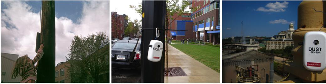
**Figure 3.9. Photographs of participant sensor placements: participant’s daughter attaching VOC sensor to street pole; and exhaust sensor outside a children’s hospital placed by activist; dust sensor attached to bridge by bicyclist.**
