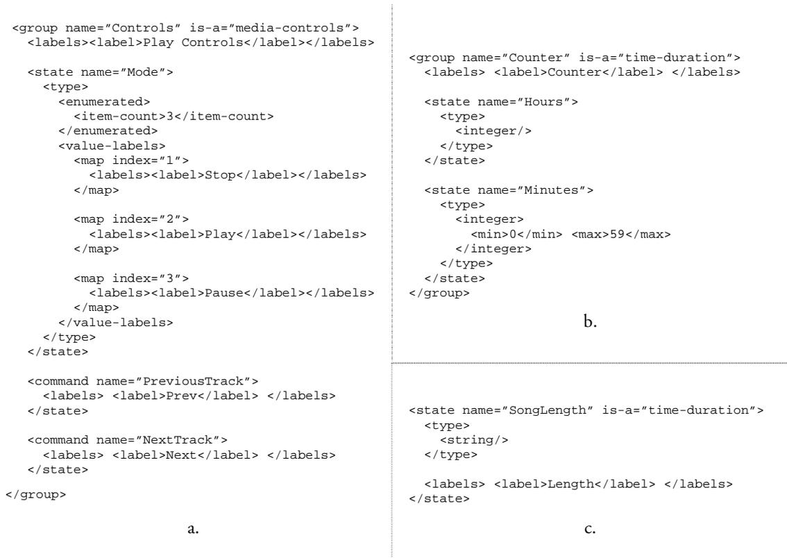
Figure 7.2. Three specification snippets showing instantiations different Smart Templates. a) The instantiation of the `media-controls` template for the play controls on Windows Media Player. b) The instantiation of the `time-duration` template for the counter function on the Sony DV Camcorder. c) The instantiation of the `time-duration` template for the song length function on Windows Media Player.
