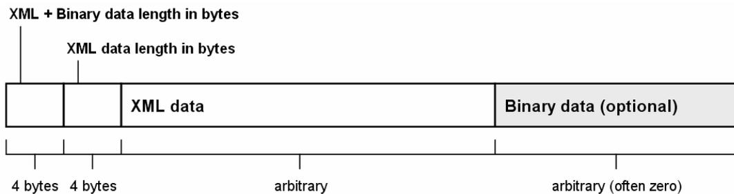
Figure 4.5. Message format for the PUC communication protocol.
