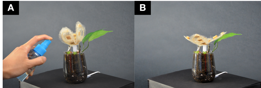
FIGURE 6.11: A custom-shaped flower made of electrospun textile and rigid plastic that actuates based on the soil's water level sensed using an electrospun liquid absorption sensor. When the soil is dry, the flower closes its petals (A). When the soil is moist, the flower actuates open.
