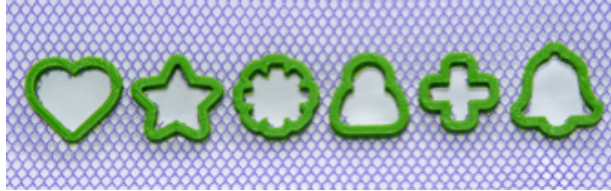
FIGURE 4.13: Custom-shaped grommets printed onto a polyester mesh. The centers of the grommets were cut out after printing.
