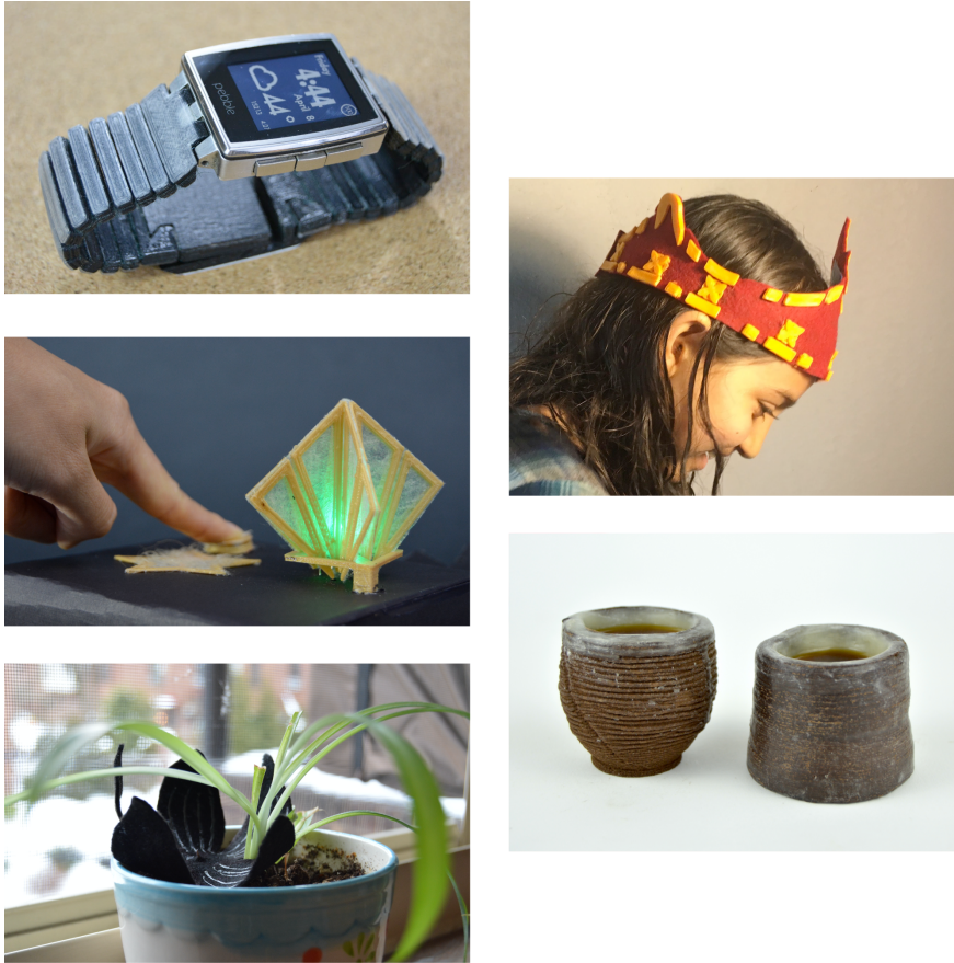
FIGURE 1.2: Examples new design possibilities enabled when combining digital fabrication techniques with everyday materials including a linked watch band with embedded textiles that absorb sweat; a custom designed crown; and origami lamp with soft input controls; a moisture-responsive plant watering indicator; and two biodegradable espresso cups made from spent coffee grounds.
