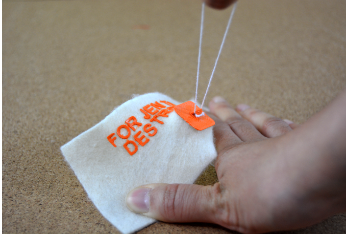
FIGURE 4.3: Plastic extruded onto a textile with a fuzzy surface creates very strong adherence. The plastic seen here is difficult to separate from a piece of felt.
