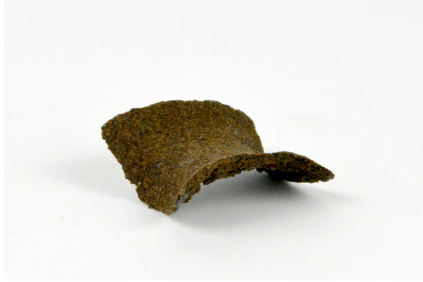
FIGURE 7.18: A single layer square printed flat with our SCG material morphed into a saddle shape as a result of shrinkage during drying.
