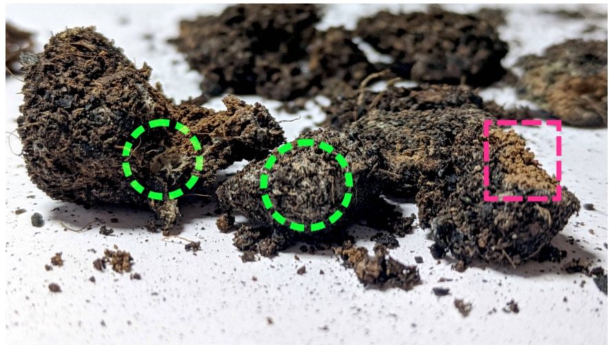
FIGURE 7.17: A few small pieces of SCG material recovered after 3 weeks of composting, distinguishable by the color of the coffee grounds highlighted in the pink rectangular outline above. The recovered pieces were brittle and showed significant mold growth (highlighted in green circles) indicating their decomposition.
