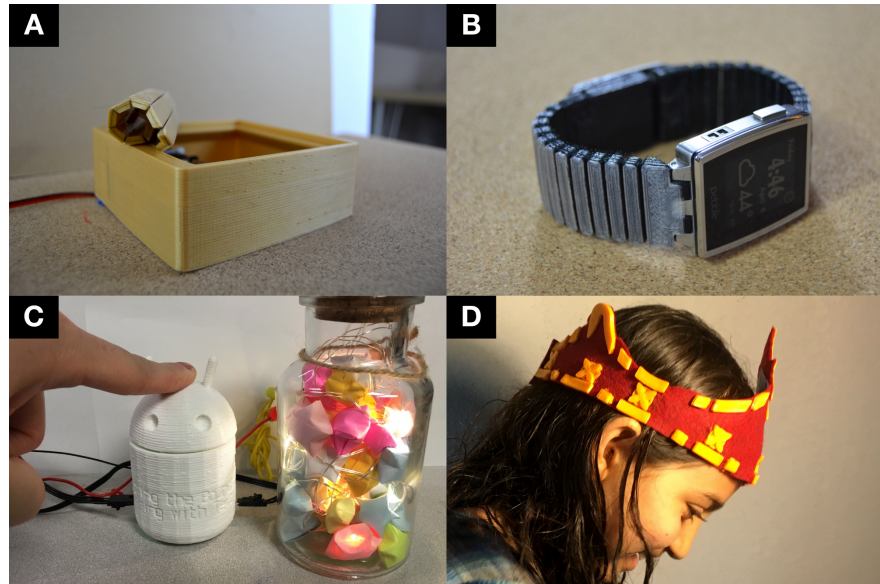
FIGURE 4.1: A range of textile-embedded 3D printed objects fabricated using our techniques—a box with a rolling lid containing a mesh of polyester and strings for actuation (A); a functional watchband printed on a polyester mesh (B); a figure with a pressure-sensitive head that controls an embedded displacement sensor containing a mesh of nylon and spandex fibers (C); a 22-inch (56 cm) crown printed on a single piece of felt that is larger than the print bed (D).
