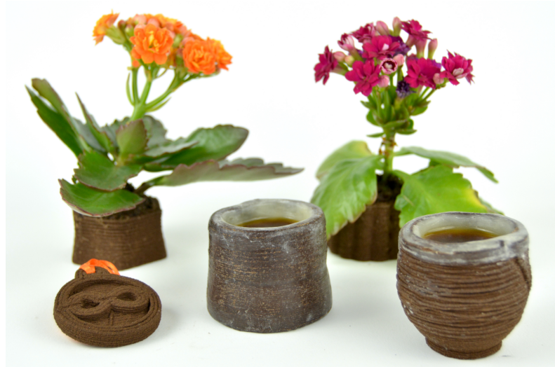
FIGURE 7.1: Examples of biodegradable objects fabricated using our new 3D printing material: an ornament necklace, two custom-shaped planter pots, and two espresso cups coated in beeswax.
