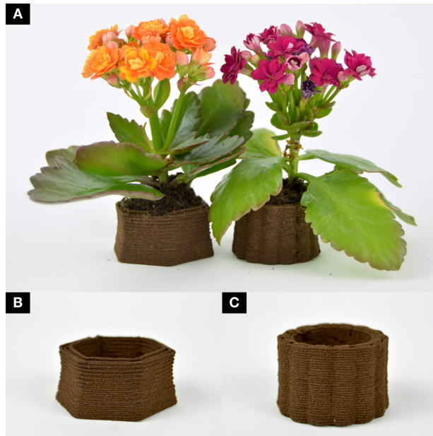
FIGURE 7.8: Biodegradable planter pots printed with our SCG material and their flowering plants (A). The first pot has a hexagonal-shape (B). The second pot is cylindrical with a ribbed pattern (C).
