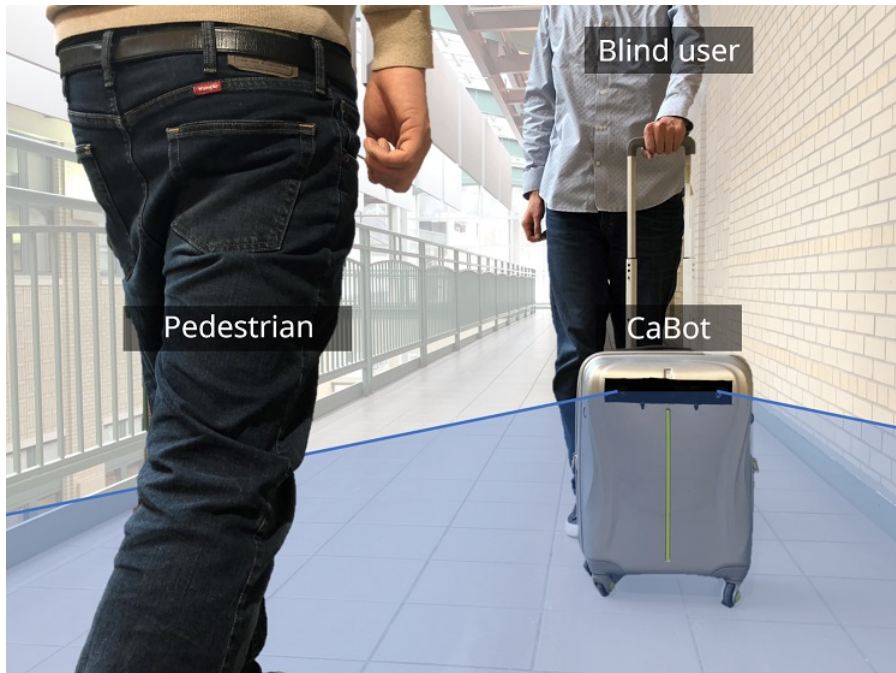
Figure 1.3: Cognitive Assistance Robot (CaBot): Our blind navigation robot leads a blind user while detecting other pedestrians and making decision of using sound alert to change pedestrians' walking direction.
