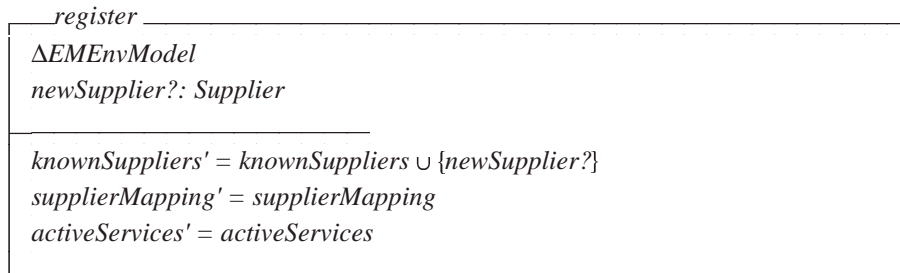
Figure 14. Z model of the effect of the register message on the state kept by the EM
