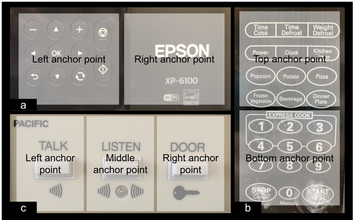
Figure 3.3: Example anchor points for different user interfaces. (a) The printer interface is divided into two anchor points, the left anchor point and the right anchor point; (b) The microwave interface is divided into two anchor points, the top anchor point and the bottom anchor point; (c) The door intercom interface is divided into three anchor points, the left, the middle, and the right anchor points.
