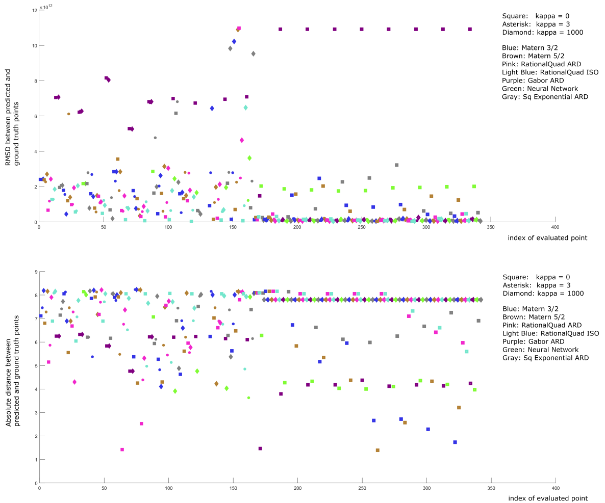
Figure 2-7: Results from 20 rounds of optimization for a large (hypersphere of radius 9 logs) search space. Individual rounds are not delineated due to variable numbers of points returned from acquisition function minimization in different rounds. Shown are (top) the RMSD values, and (bottom) the errors in predicted parameter sets as the search progresses. Note that the best points found (very low RMSD) often correspond to comparatively distant parameter sets. This is a result of the fact that the objective can be insensitive to large displacements in some of the input dimensions but not others.
