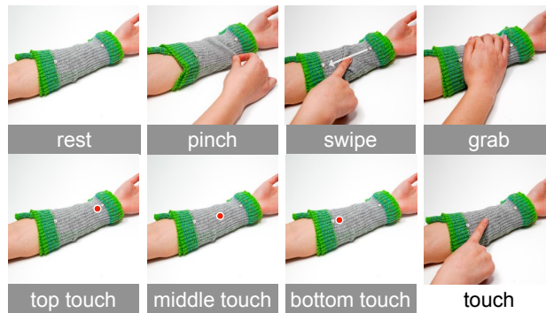
Figure 21: The seven gestures used for Study 2. Touch was performed at three different points(indicated by the dots), shown in the bottom row.
