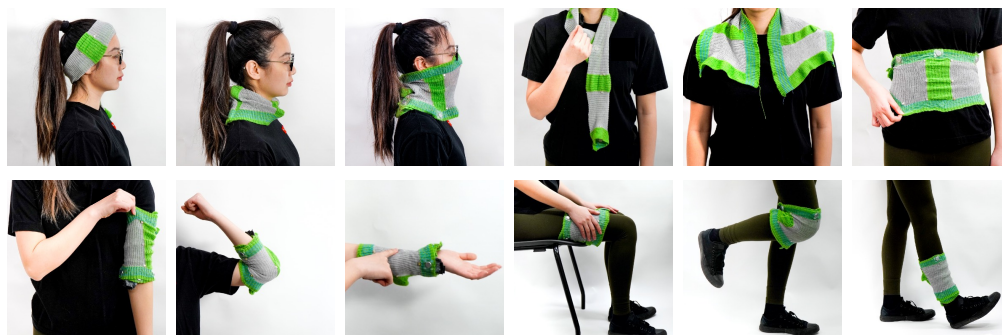
Figure 12: uKnit is a scarf-like reconfigurable wearable which can recognize its current body location placement and perform a variety of gesture recognition and sensing tasks.
