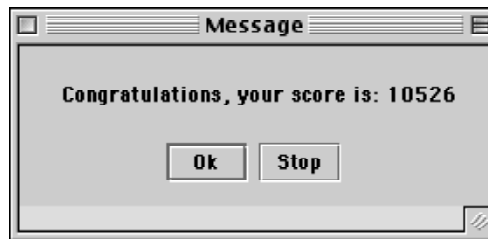
Figure 5-6. A dialog box similar to this will come up when the statement tell "Congratulations, your score is:", score's back is executed. Execution pauses while the dialog box is showing. If the Ok button is pressed, execution continues; if the Stop button is pressed, the program is halted.
