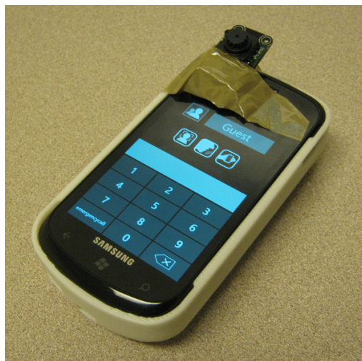
Figure 5.3 The prototype used to test the authentication methods. The casing on the rear side of the phone contained a Gadgeteer and a touch sensor.
