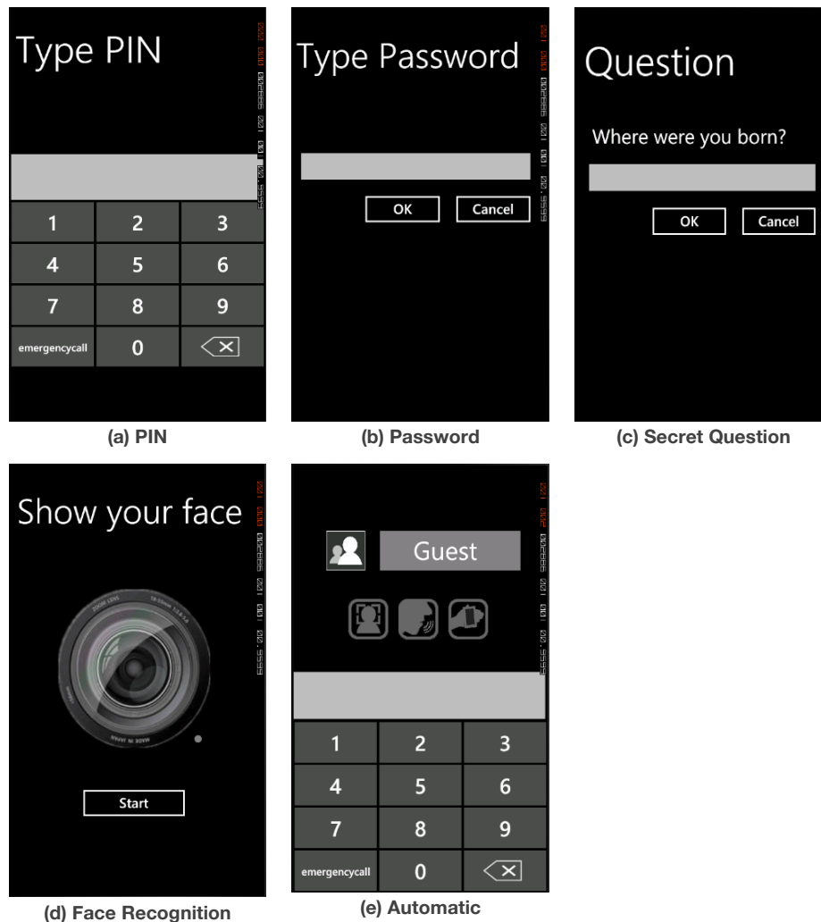
Figure 5.4 The screens presented in each of the five authentication methods we tested.
