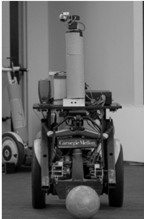
Figure 4.15: The Segway RMP soccer robot equipped with a kicker, a catcher, infrared sensors, and a camera mounted on a custom pan-tilt unit.
